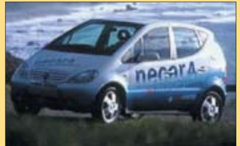
The new car is powered by a fuel cell, which generates electric power from hydrogen. Singapore will provide the necessary infrastructure for alternative fuel cell vehicles, vehicle operation and maintenance.
